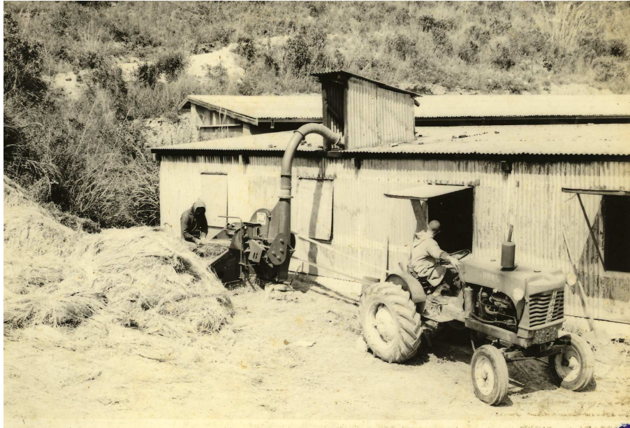
圖片(37)： 圖中央的機器是將乾草切成碎塊，作為牛隻的食料。 The machine in the centre is for grinding the straw into pieces which are used to feed the cows.
